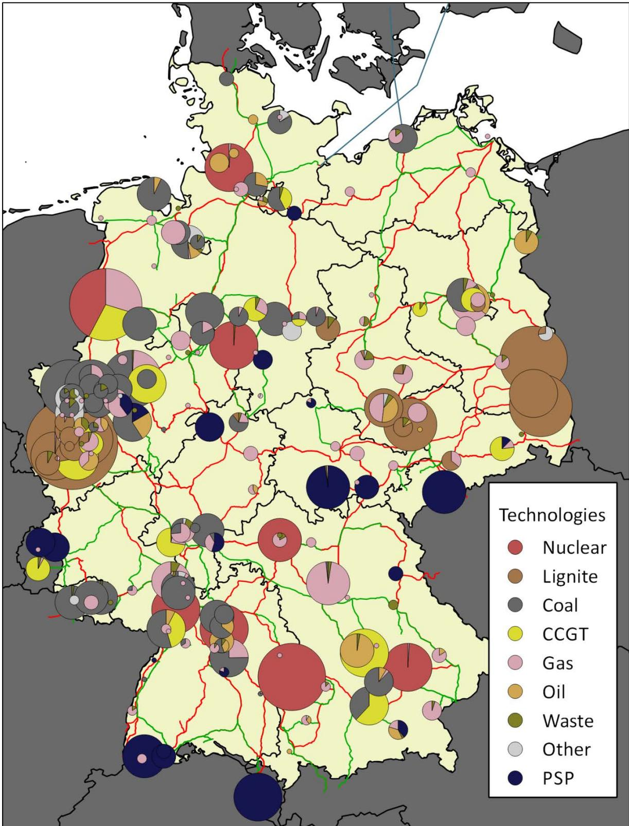
**Figure 11: Conventional generation capacity on a nodal level**
