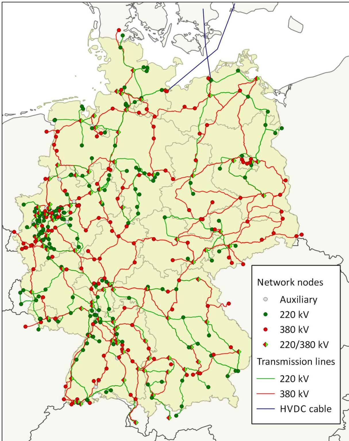
**Figure 4: The German high-voltage electricity transmission system in 2012**
