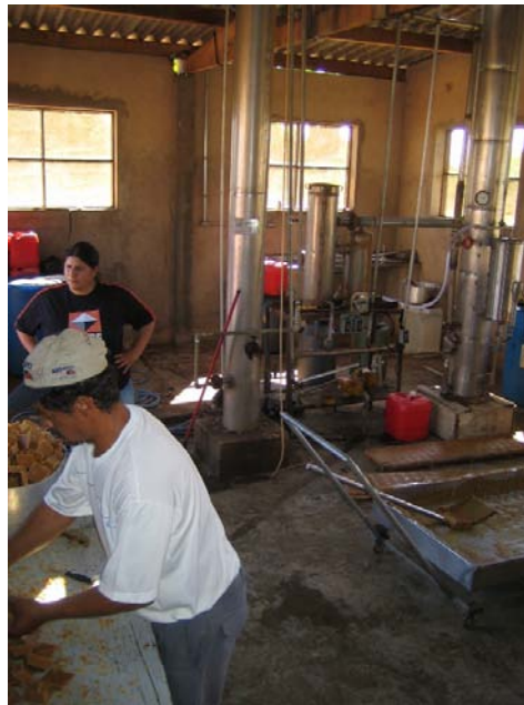
Production of rapadura sweet (left margin) and mini-distillery for ethanol (background) in Angatuba
