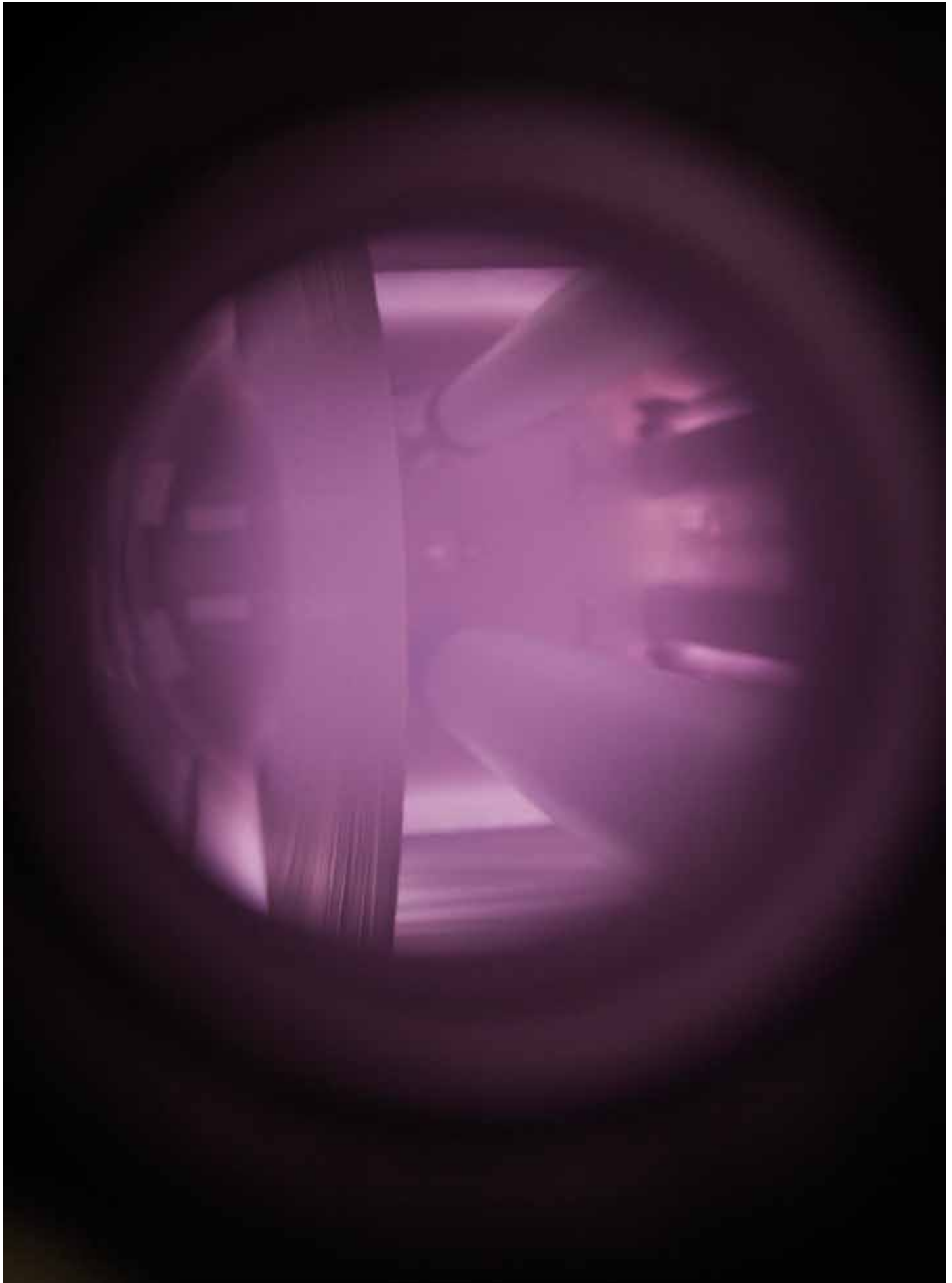
View inside a low-pressure plasma reactor at the Fraunhofer IFAM's PLATO section. © Dirk Mahler, Fraunhofer Institute for Manufacturing Technology and Advanced Materials IFAM.
