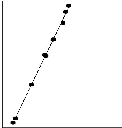
Figure 1: *Illustration of additive measurement error model.* The filled circles are the true  $(\mathbf{Y}, \mathbf{X})$  data and the line is the least squares fit to these data. For these data  $\sigma_x^2 = \sigma_u^2 = 1$ ,  $(\beta_0, \beta_x) = (0, 1)$  and  $\sigma_\epsilon^2 = .25$ .
