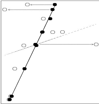
Figure 2: *Illustration of additive measurement error model. The filled circles are the true  $(\mathbf{Y}, \mathbf{X})$  data and the steeper line is the least squares fit to these data. The empty circles and attenuated line are the observed  $(\mathbf{Y}, \mathbf{W})$  data and the associated least squares regression line. For these data  $\sigma_x^2 = \sigma_u^2 = 1$ ,  $(\beta_0, \beta_x) = (0, 1)$  and  $\sigma_\epsilon^2 = .25$ .*
