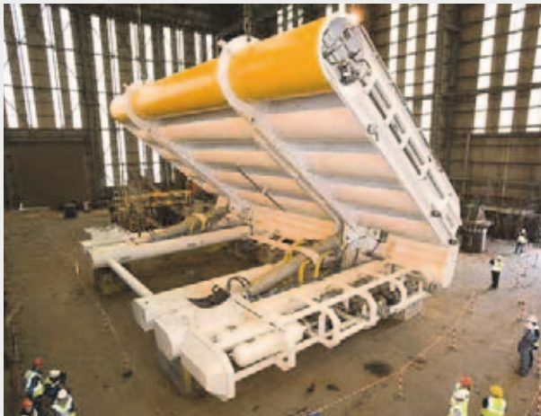
System components of Oyster Wave Energy Converter (Source: Aquamarine Power)
