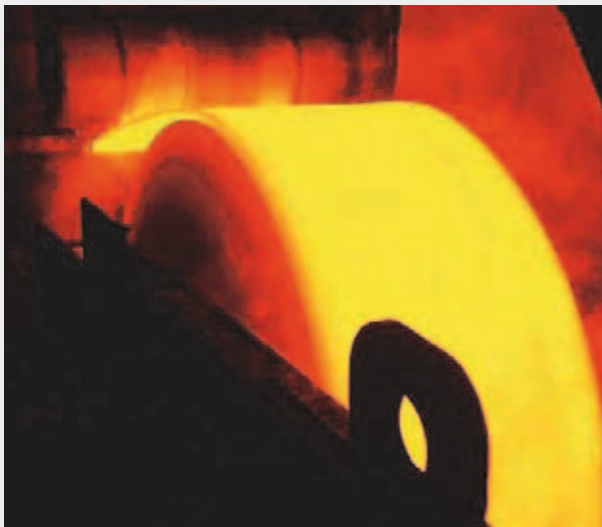
Coiling of the casted steel strip (Source: Salzgitter Mannesmann Forschung GmbH)
