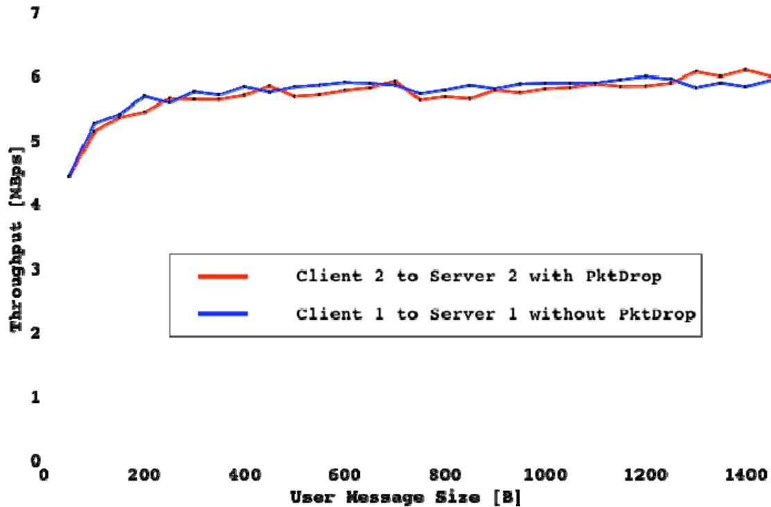
Figure 9: Throughput of the bottleneck link, if the link between Client 2 and Router 1 is configured with an error rate
