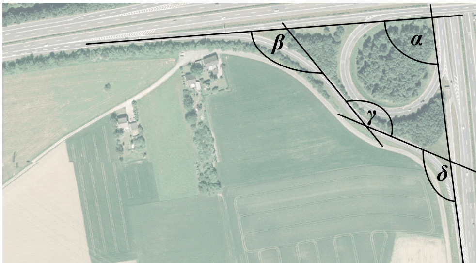
Figure 5: Determination of the angles on a ramp
