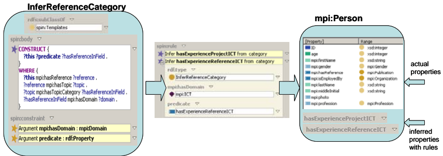
Figure 5: Extension of the conceptual class and property schema with rules
