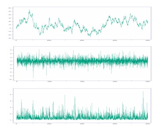
Figure 1: The simulated compound-Poisson driven COGARCH(1,3) process with jump-rate 2, normally distributed jumps with mean zero and variance 0.74 and coefficients  $\alpha_0 = \alpha_1 = 1$ ,  $\beta_1 = 1$ ,  $\beta_2 = .48 + \pi^2$ , and  $\beta_3 = .64 + .4\pi^2$ . The graphs show the process  $(G_t)$  sampled at integer times (top), the corresponding increments  $((G_{t+1} - G_t))$  (centre), and the corresponding volatility sequence  $(\sigma_t^2)$  (bottom).
