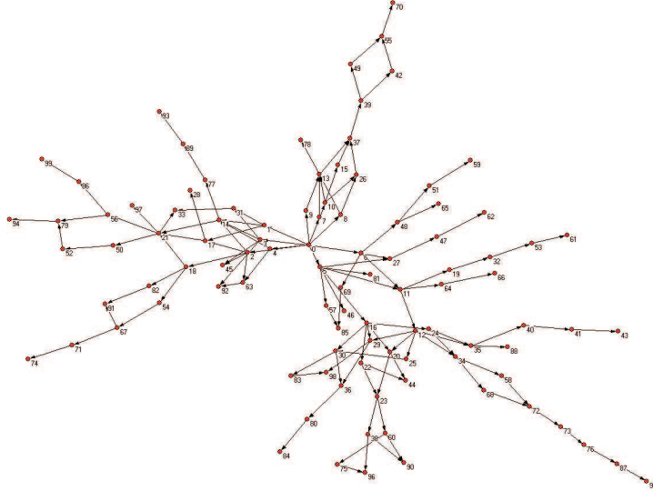
Figure 1: PT Network: N^{nodes} = 100 , InitialNodes = 10 , P^{split} = 25\%
