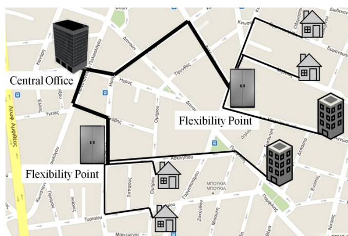
Figure 1. FTTH access network architecture
