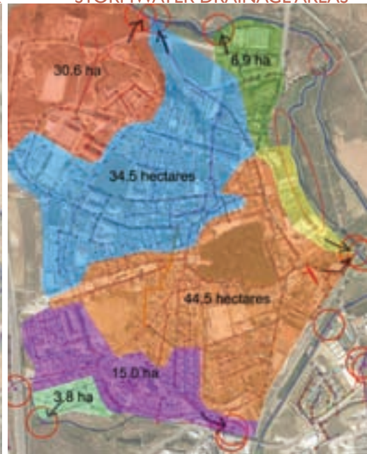
STORMWATER DRAINAGE AREAS
