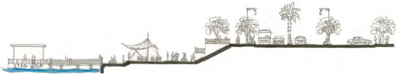
FIGURE 146. Proposed section C-C': Landscaped ferry terminal with benches and services for passengers
