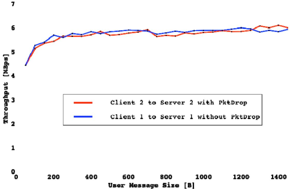
Figure 9: Throughput of the bottleneck link, if the link between *Client 2* and *Router 1* is configured with an error rate
