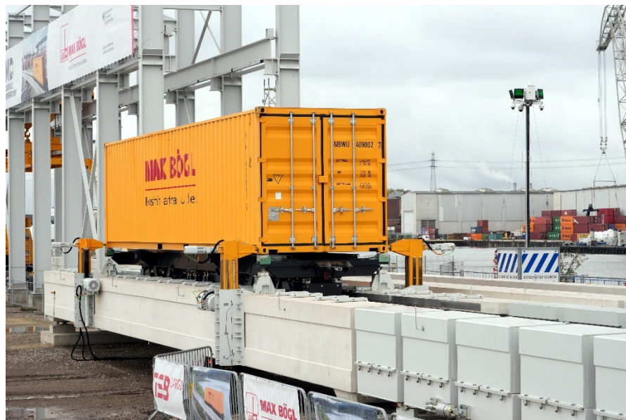
FIGURE 9d: The Transport System Bögl (TSB) for cargo transportation [7].
