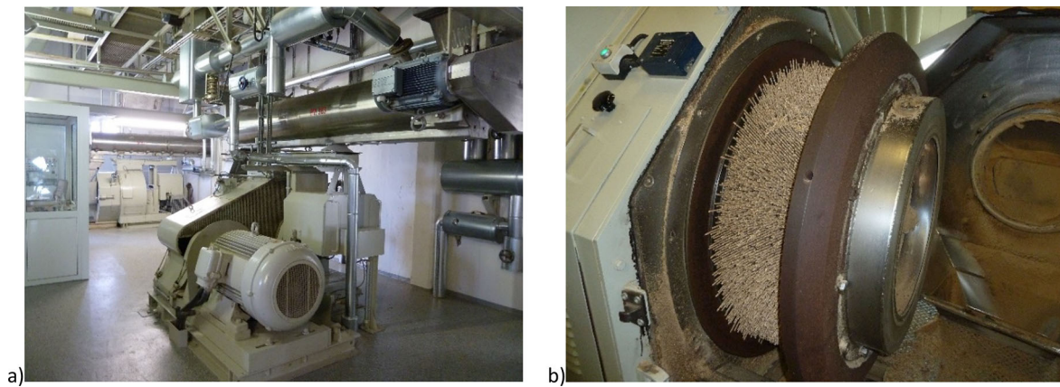
Fig. 2 Images of the press machine modeled in this study. The machine is used in the pelleting process of compound feed production. a Shows the complete press machine, and b the inner matrix where the compound
