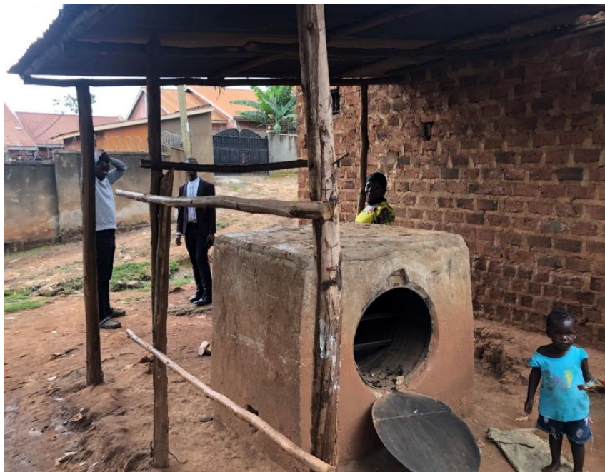
Figure 11: Photo of an oven used for meal cooking and for hot air pasteurization of mushroom substrate in Uganda. Firewood is used to heat the metal drum, which is embedded in a clay structure.
