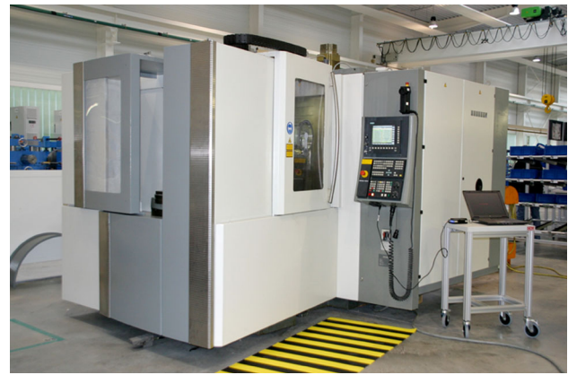
Fig. 12 DMC-50H CNC-milling machine used as a test bed within the CiP-DMD dataset
