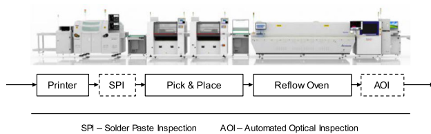
Fig. 7 Process chain for PCB assembly (picture by (Kitchenham et al., 2009))
