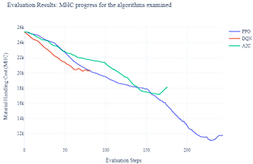
Fig. 8 Evaluation result of training three RL algorithms on the instance P12 for 1M steps each. It can be observed that PPO yields the best results given identical hyper-parameters as it achieves the lowest MHC
