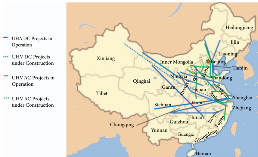
Figure 7.6 China's UHV-DC and UHV-AC power grid, 2020
