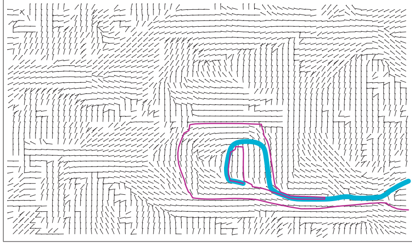
Figure 1: Examples of tracks generated by Algorithm E (narrow line) and Algorithm T1 (wide line) for \Delta t = 0.1 with the same starting point and without random noise ( \sigma = 0 ).
