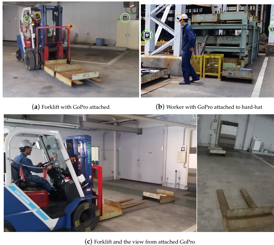
Figure 18. Experiment conducted with workers and forklifts (movers) at indoor and outdoor locations at Tsuneshi shipyard in Hiroshima prefecture, Japan. (a) GoPro wireless cameras attached to the worker and forklift (highlighted in orange). Static markers to determine observer location with respect to the environment (highlighted in green). (b) Worker with GoPro attached to hard-hat (orange highlight) interacting with a stack of workpieces gets located within workspace through static markers in the environment (green highlight). (c) Movers (forklift) picking up a workpiece (left) and the point of view from the camera attached to the forklift (right).
