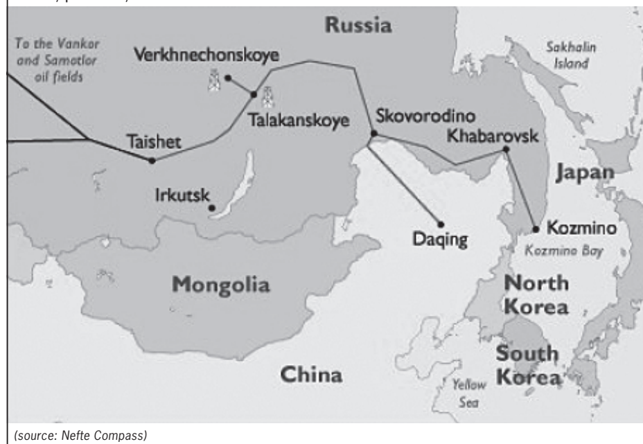
Map 1: The ESPO pipeline: phase 1, Taishet to Skovorodino and spur to Daging in China; phase 2, Skovorodino to Kozmino.
