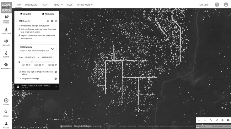
Figure 5.2 Screen capture of GFW with RADD alerts in the Central African Republic based on Radar data by Sentinel 1 within 10-meter pixels. The lines indicate recent logging in a typical grid-like structure along roads.
