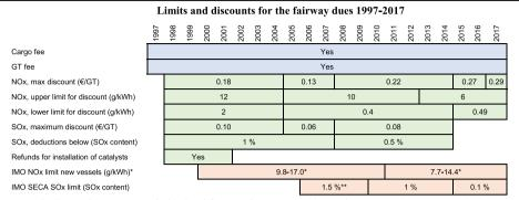
Notes: \* The maximum NOx emission level for vessels constructed in or after 2000 and 2011, respectively. The specific level (within the interval) is dependent on the engine speed (IMO, 2017b); \*\* The SECAs were in effect from May 2006 in the Baltic Sea and November 2007 in the North Sea (IMO, 2017c).
