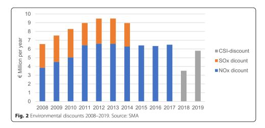
of calls with a discount for RoRo-vessels (from 3% in 2017 to 41% in 2019) and tankers (from 1% in 2017 to 11% in 2019). Owners of container vessels did not undertake any measures to receive discounts, neither in the NOx-certificate based system nor in the CSI-based system.
