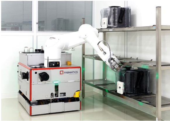
Figure 2: Multiple-load AGV equipped with a robot arm handling at a shelf in a semiconductor production facility (reference: www.fabmatrics.com )
