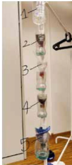
Fig. 1 To illustrate the wastewater treatment process created by using transparent plastic bottle
