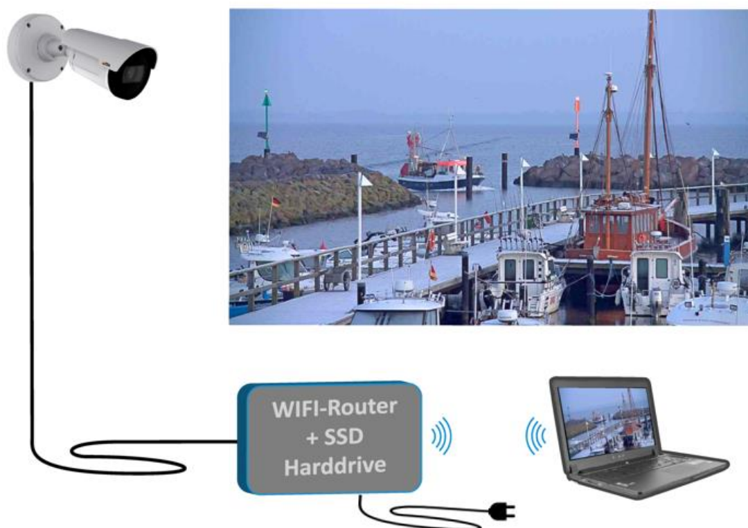
Fig. 9: Setup of the remote camera systems used to monitor the recreational salmon trolling effort around the Island of Rügen.
