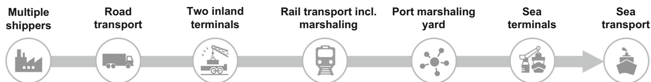
Fig. 2 Intermodal container transport chain from the shipper to sea transport
