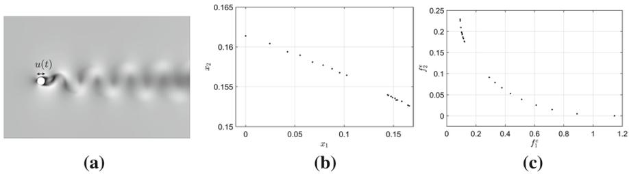
**Fig. 9** **a** Flow around a cylinder, controlled via cylinder rotation. **b** Result of the weighting method applied to the MOP (19) in the variable space. **c** Image of the resulting points under the objective function (19)
