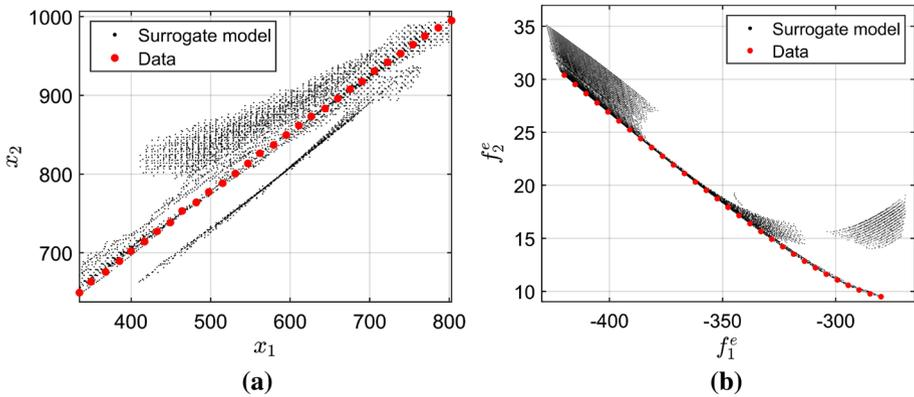
**Fig. 12** **a** Projection of the Pareto critical set of the surrogate model and the data that was used to create it for Example 8. **b** Image of the Pareto critical set of the surrogate model and the data under the original objective function vector
