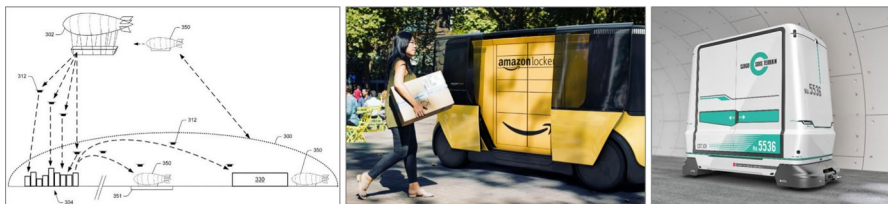
Fig. 9 Patent drawing for flying warehouse (left; Source : Berg et al. 2016), mobile parcel locker called Hannah (middle; Source : Teague 2020), and tunnel-based cargo transport with an automated guided vehicle (right; Source : CST 2020)
