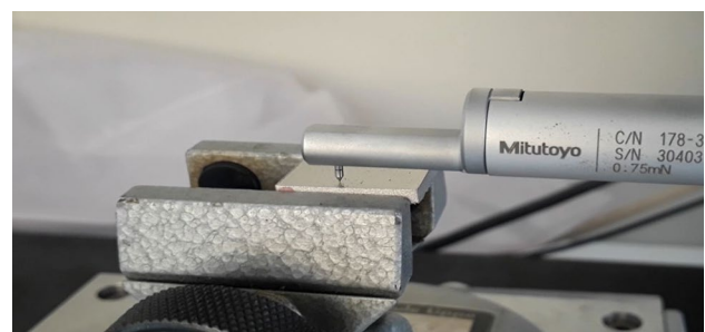
Fig. 5 Surface roughness measurement via a stylus instrument
