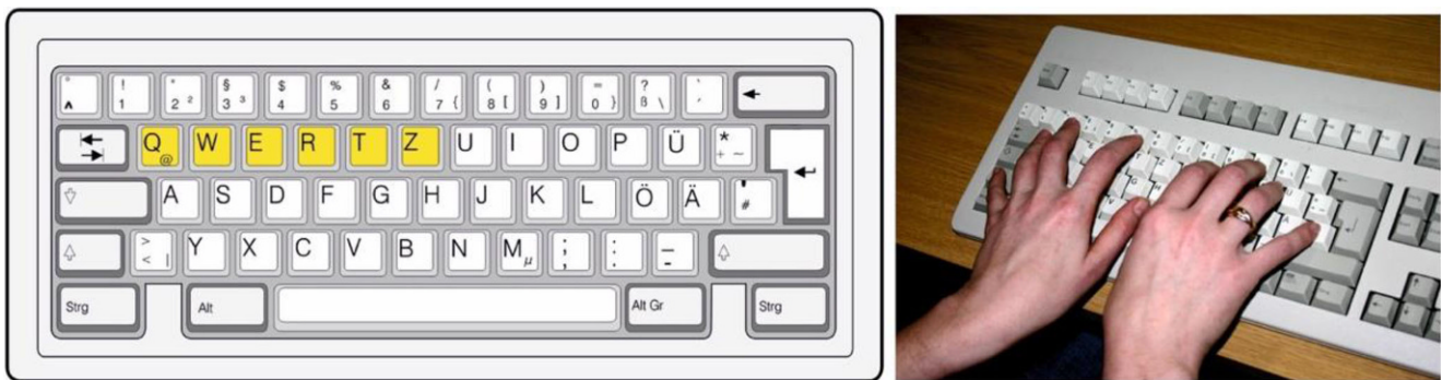
Fig. 6 Conventional QUERTZ-Keyboard (DIN EN 2137-2 1999) demanding inward rotation (pronation) of the forearm and ulnar deviation of the hand—an unnatural posture due to the parallel arranged rows of a keyboard
