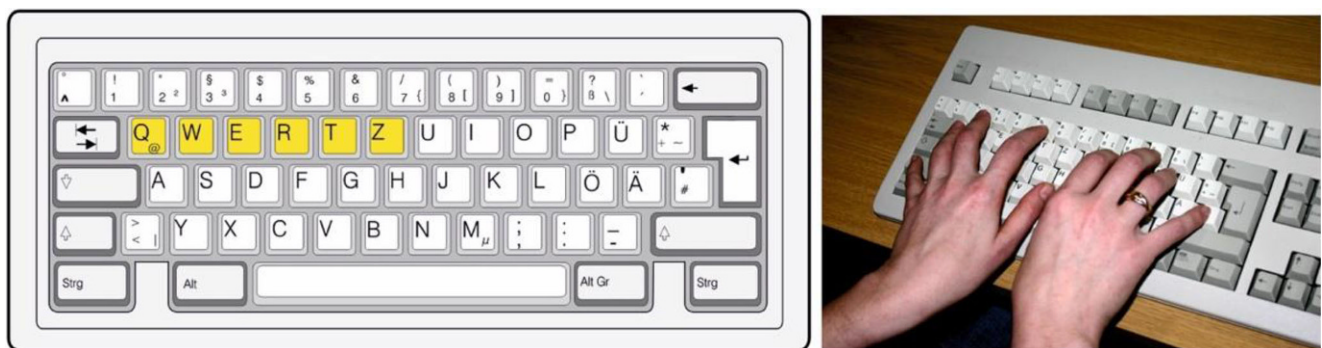
Fig. 6 Conventional QWERTZ-Keyboard (DIN EN 2137-2 1999) demanding inward rotation (pronation) of the forearm and ulnar deviation of the hand—an unnatural posture due to the parallel arranged rows of a keyboard
