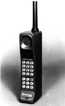
Lightweight, portable subscriber units for the Iridium system communicate directly with satellites, using a small antenna.
