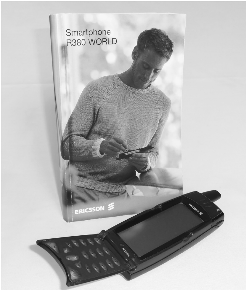
7.7 The Ericsson R380 World smartphone. Developed in Sweden and introduced in late 2000, the smartphone used dual 900/1800 GSM standards. Combining a mobile phone with a PDA, when opened, the whole screen could be used as a PDA using a touch sensitive keyboard or a stylus to enter text. The R380 was the first smartphone to use the Symbian operating system. Courtesy Nigel Linge and Andy Sutton.
