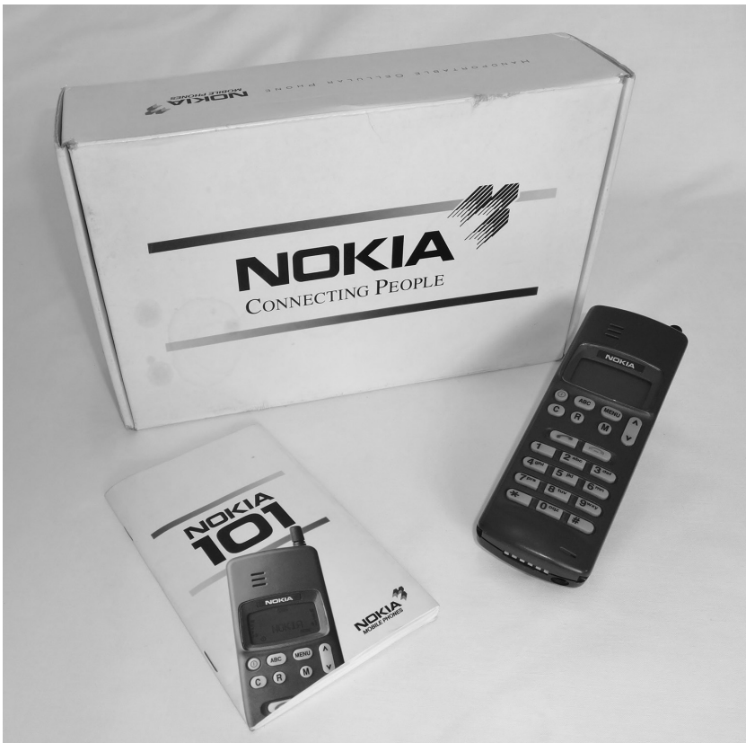
3.2 The Nokia 101, introduced in 1992. It was one of the last handsets of the analog era. With its “candy bar” form factor, it claimed to be the world’s most portable phone. Courtesy Nigel Linge and Andy Sutton.
