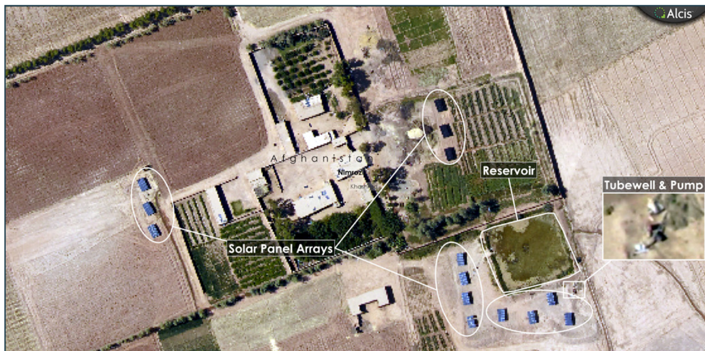
Figure 7 Imagery showing the use of solar powered deepwells in former desert areas of Khashrud
