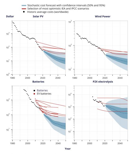
Stochastic cost forecasts for solar PV and wind power (generation costs) and batteries (capacity costs) in a fast energy transition scenario based on Way et al. (2022). None of the scenarios by the International Energy Agency (IEA) or the Intergovernmental Panel on Climate Change (IPCC) is depicting the trends that can be expected.
