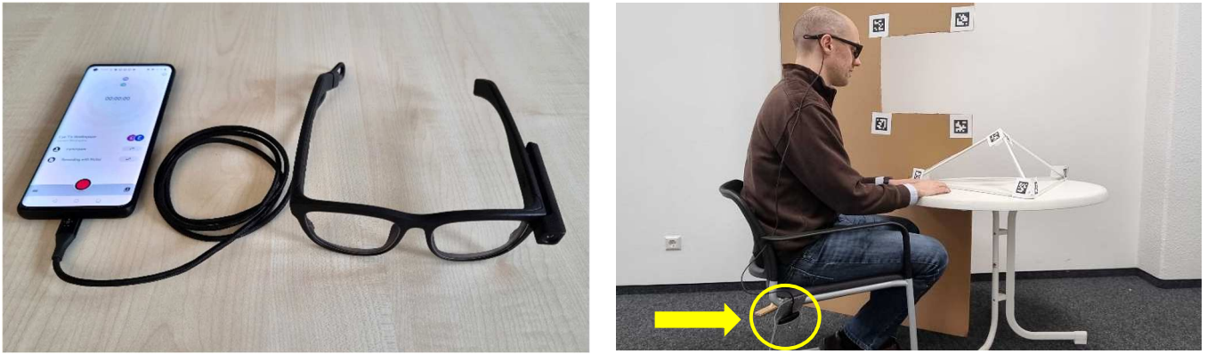
Figure 3. Illustrated is a Pupil Invisible connected to the Pupil Labs Companion Device (left) and a participant equipped with both devices (right). During the non-binding communication stage, the mobile phone was stored in a small pocket (yellow circle) attached to the chair so that it would not interfere with the real effort task.
