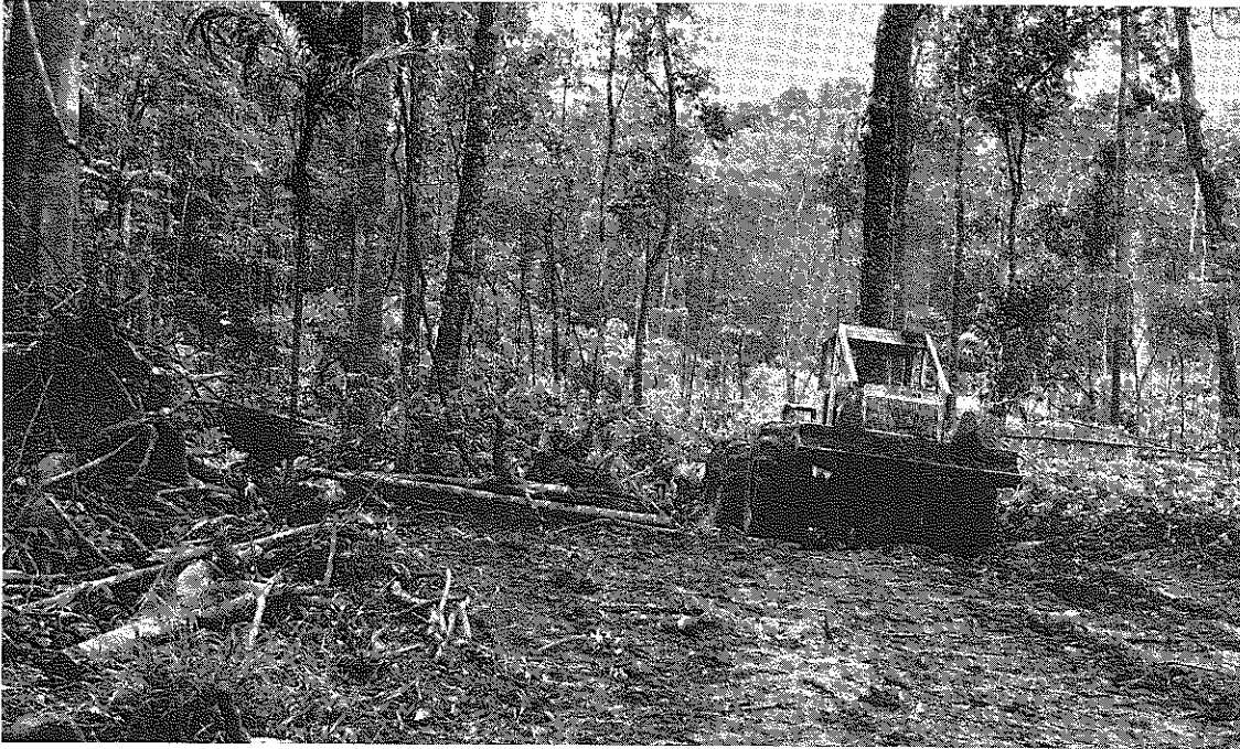
A skidder drags a log out a forest trail to the nearest road. As much valuable timber as possible has been sold before the land is cleared for agriculture. The density of any particular species is very low, so most of it has been sold as undifferentiated hardwood.
