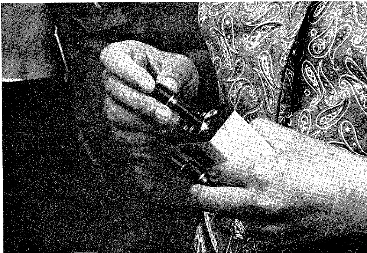
FIGURE 7. INSERTION OF E-CELLS PRIOR TO MONITORING
