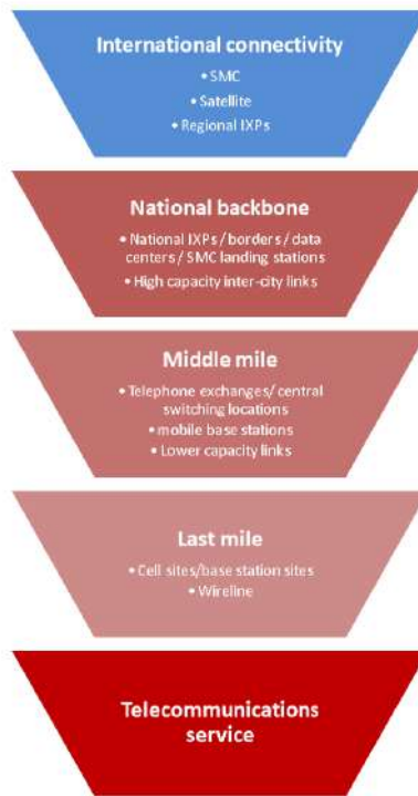
Figure 2: Internet access value chain and key telecommunication infrastructures.
