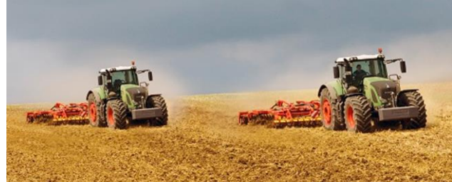
Figure 7: Fendt GuideConnect – Two Tractors, One Driver
