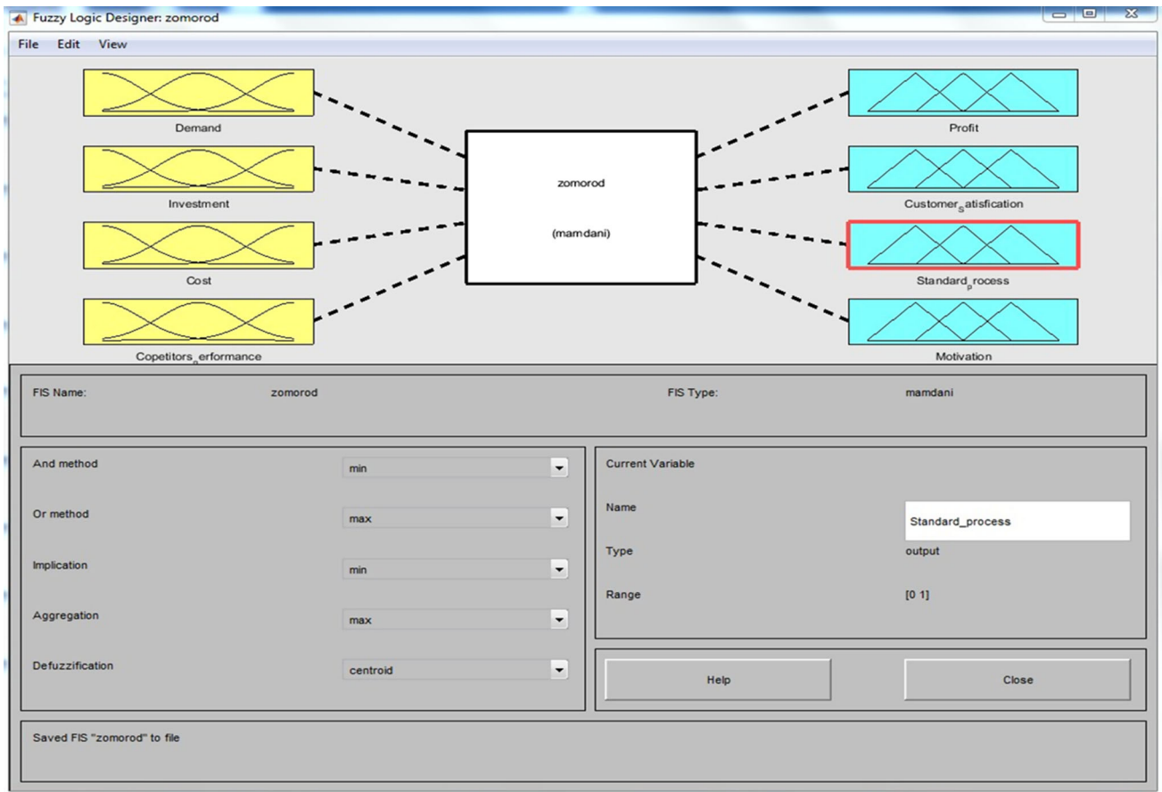
Fig. 2 Outline of inputs and outputs in fuzzy Mamdani operator
