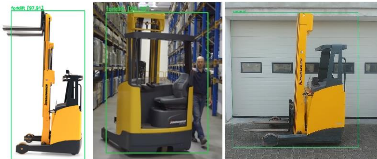
Figure 14: Forklift detection results with good impression
