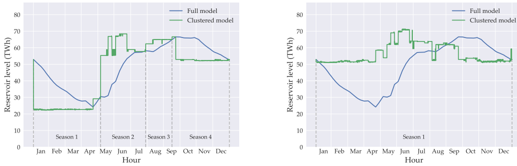
(a) Model til K=25 states and 3 seasonal splits (b) Model with K=30 states and no seasonal splits
