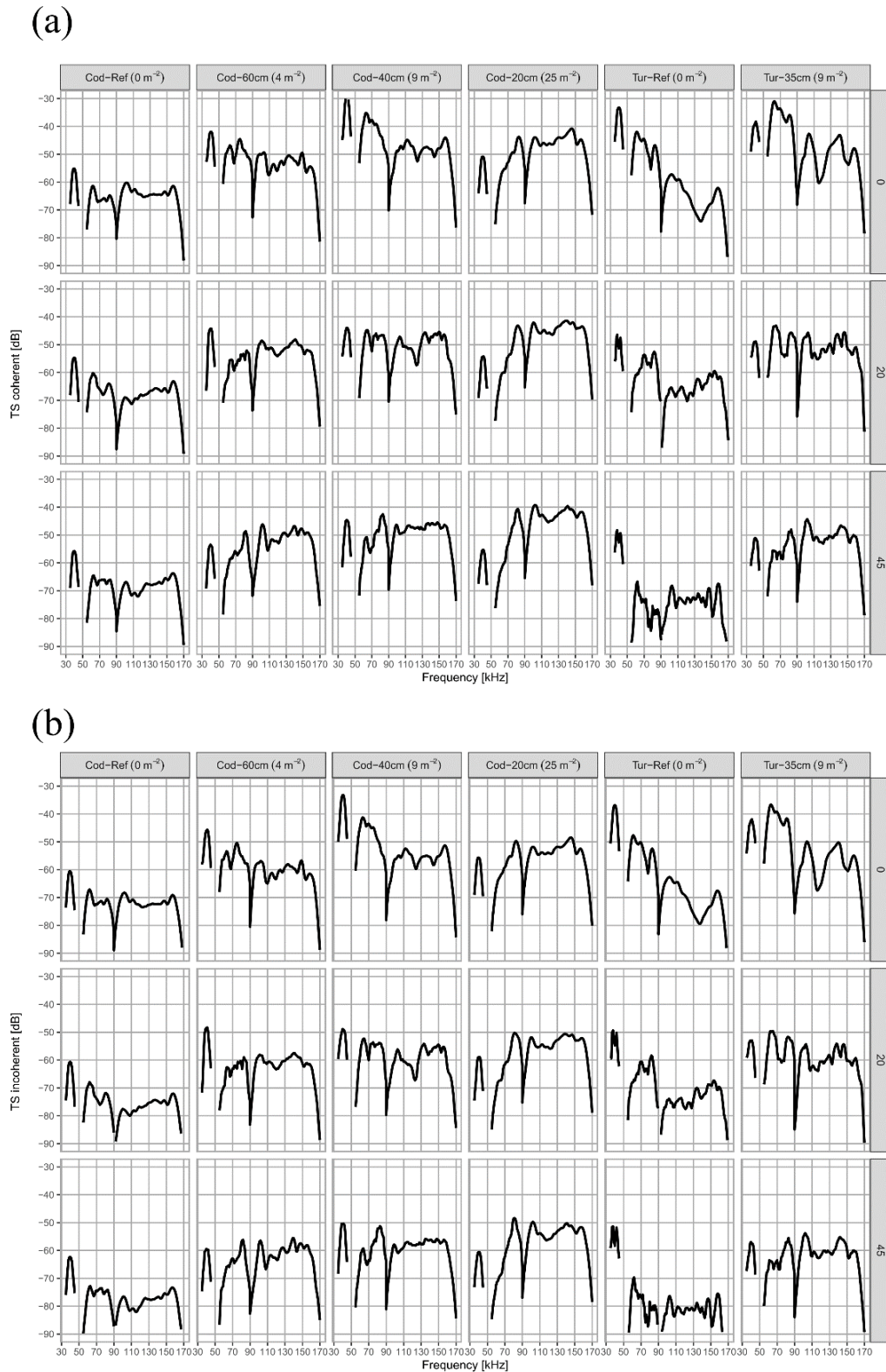
FIGURE 10: Mean coherent (a) and incoherent (b) TS vs frequency for each unique combination of net type and inclination; number of sphere/m 2 provided in brackets. SD is not shown for clarity, but given in the appendix (FIGURE A. 4; FIGURE A. 5). Raw data available in the supplementary material. Data on the edge of the measurable frequencies (55 kHz, 90 kHz and 170 kHz) should be treated with caution and is not used in the further analysis.
