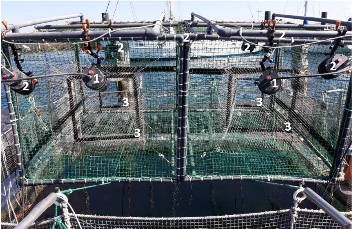
Fig. A4. Experimental pot with two exchangeable entrances. Two IR cameras (1) in front of each funnel entrance and two IR lights (2) on each entrance side (one inside above the funnel inner opening, the other outside next to the IR cameras). Black frames around funnels are RFID antennae (3). Note: Owing to technical difficulties, RFID data could not be used in the data analysis.
