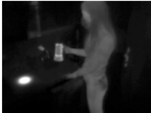
Figure 17. Raw thermal image showing a switched-on stove and a person in the kitchen
