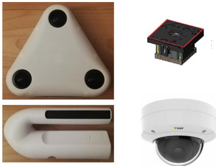
Figure 12. Different camera types used in AAL applications: top left - Omnidirectional camera, top right - Thermal camera, bottom left – depth sensor, (d) bottom right – RGB dome camera.
