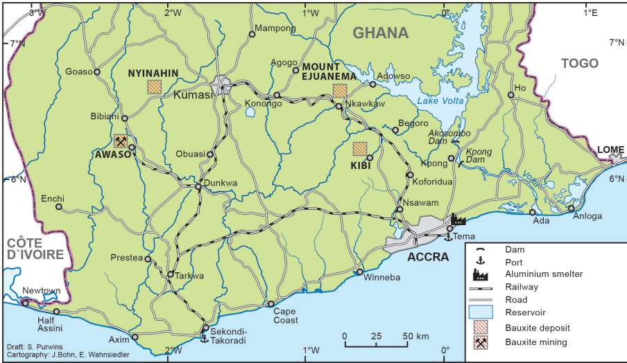
Fig. 1: Infrastructure of the bauxite-aluminium industry in Ghana
