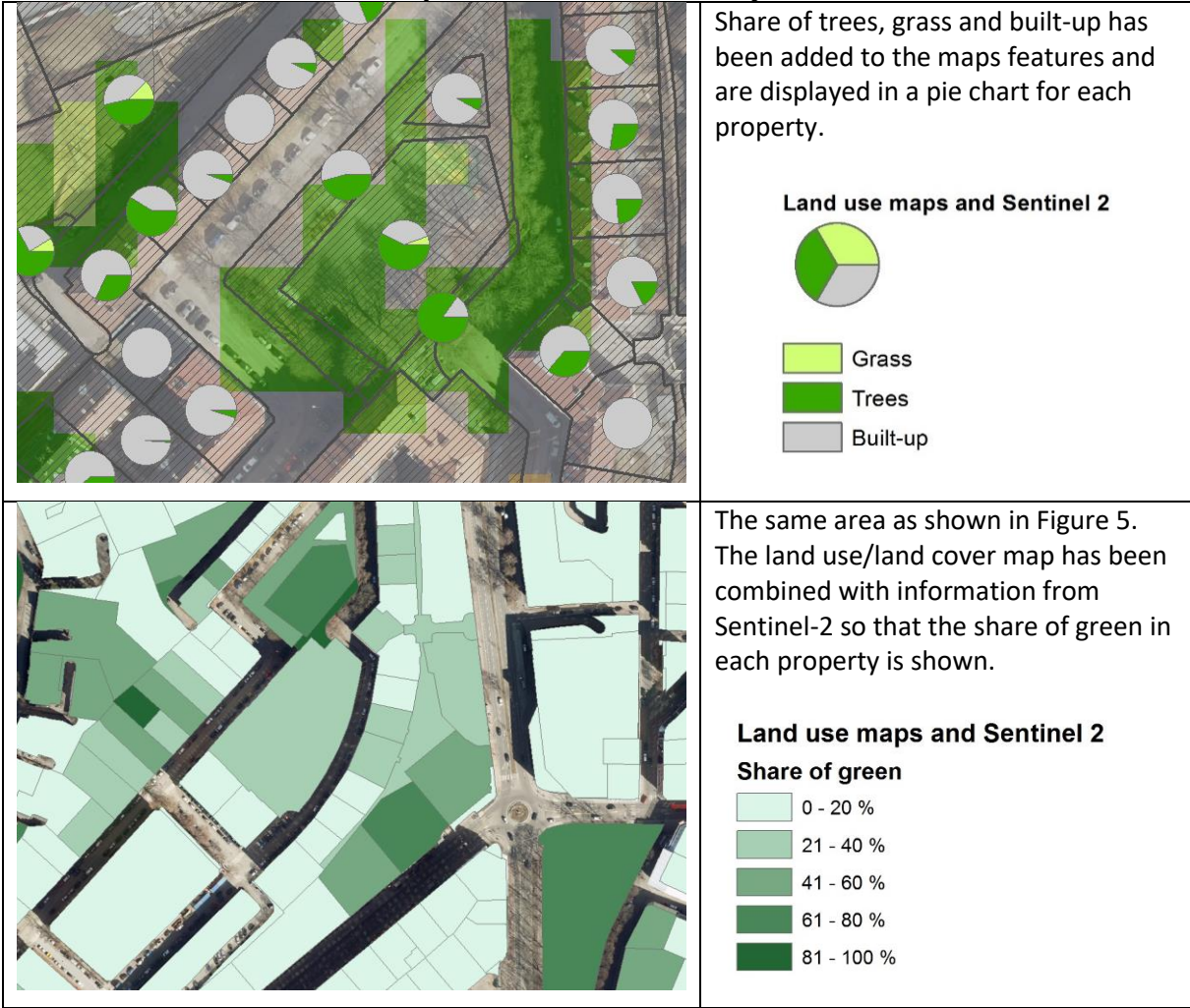
Figure 12. Proportion of Sentinel-2 classes visualized using intersection of Sentinel-2 landcover classification and Statistics Norway’s land use/land cover map
