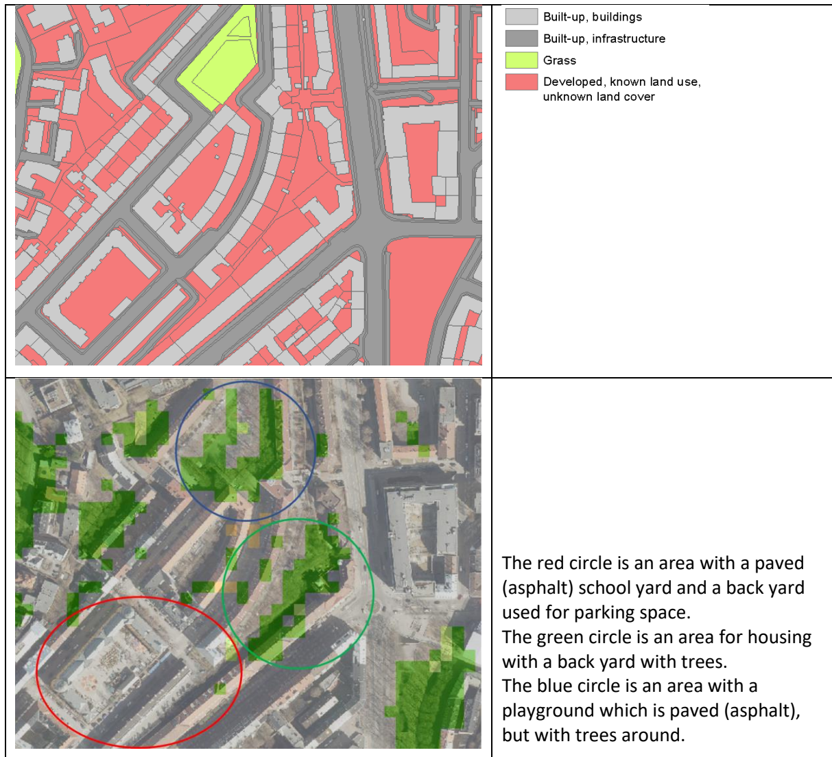
Figure 5. Principle for combination of Statistics Norway land use/land cover maps and Sentinel-2 land cover classification (raster map). Example from a case study area (Akersveien)
