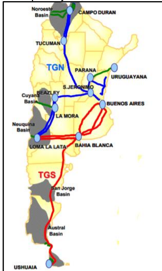
Figure 19: Argentine Domestic Pipeline System
